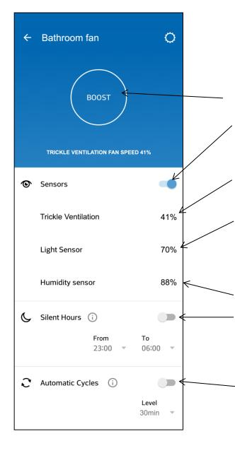
Manually boost the fan for 15 minutes at any time to apply maximum ventilation.
